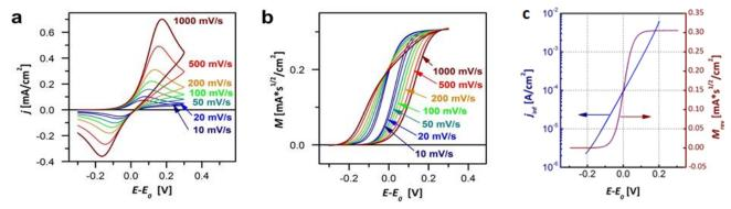
Simulated CVs of a diffusion affected charge transfer reaction with varied scan rates (a), their semiintegrals (b), and the calculated  $j_{inf}$  and  $M_{rev}$  functions (c). Simulation parameters:  $D_{red} = D_{ox} = 10^{-5}$  cm<sup>2</sup>/s,  $c_{red} = 10^{-6}$  mol/cm<sup>3</sup>,  $c_{ox} = 0$  mol/cm<sup>3</sup>,  $E_0 = 0$ ,  $k_0 = 0.001$  cm/s,  $\alpha = 0.5$ .
